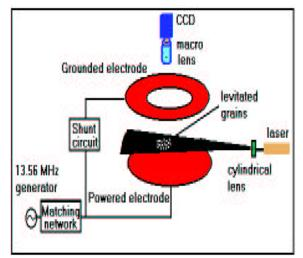
Figure.4. Schematic of the typical experimental setup used for the generation of plasma crystal in RF plasma.
